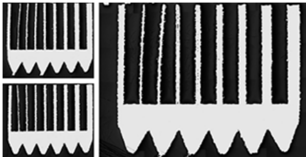
Fig 8: Thin wall samples - thickness range 0.15 - 1mm
