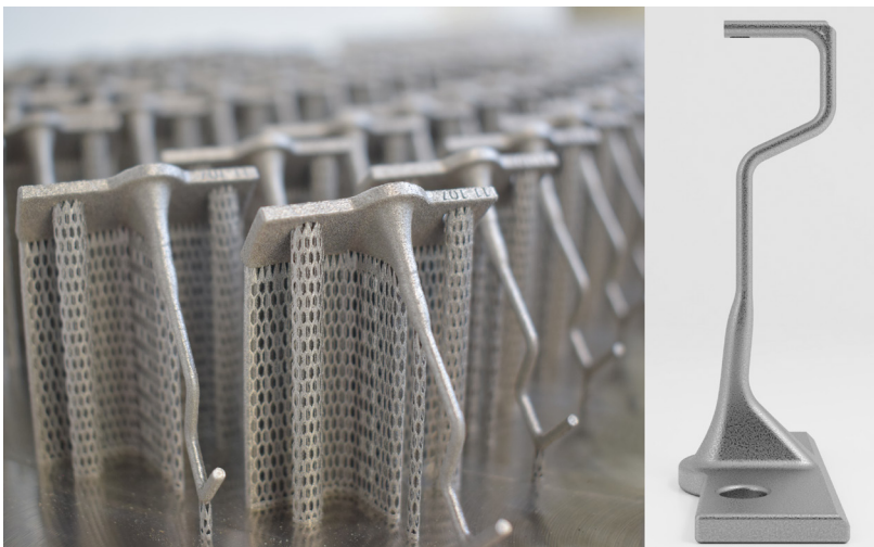
Figure 8. Nozzle parts as built in MetalFab
