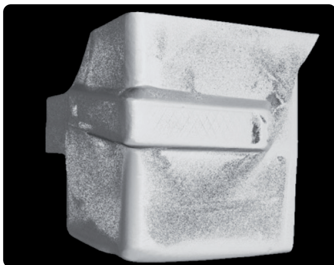
CT scan of printed Chassis Inserts
