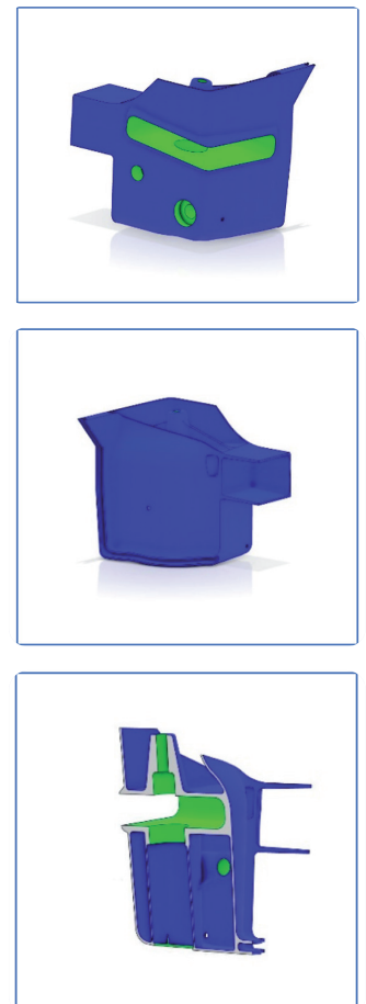
CAD views of front suspension chassis insert
