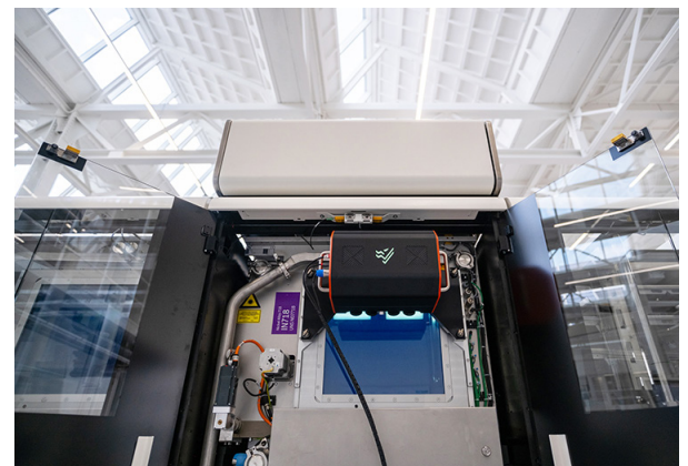
Fig 1: Setup of AMiRIS hardware in MetalFab system
