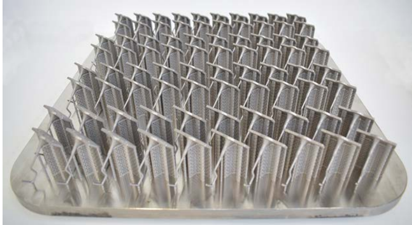
Figure 7. The M789 tooling nozzle build manufactured with MetalFab
