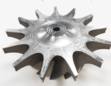
Figure 7. Machined base profile
